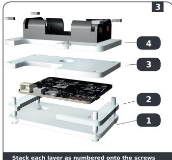
Stack each layer as numbered onto the screws through layer no. 1, then tighten nuts.
