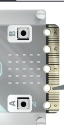
MI: protective case for the BBC micro:bit. It's 4 - layer construction is easy to assemble and gives access to all ports and buttons. It also allows for use with breakout boards and crocodile clips without having to remove the BBC micro:bit!
