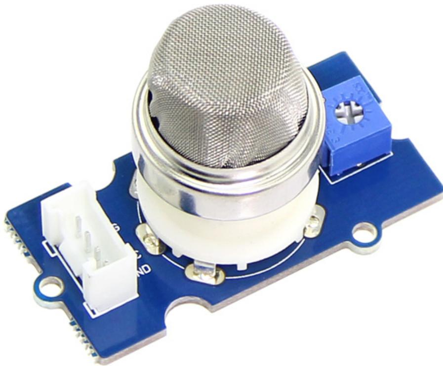
The Grove - Gas Sensor module is useful for gas leakage detecting (in home and industry). It can detect LPG, i-butane, methane, alcohol, Hydrogen, smoke and so on. Measurements can be taken as soon as possible based on its fast response time. Also the sensitivity can be adjusted by the potentiometer.
